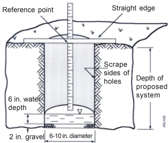
Figure 2. Typical cross-section of a perc test hole.
