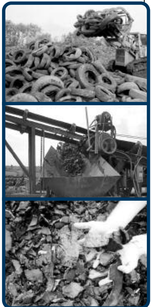
Problematic discarded tires can be turned into useful drainfield media.
